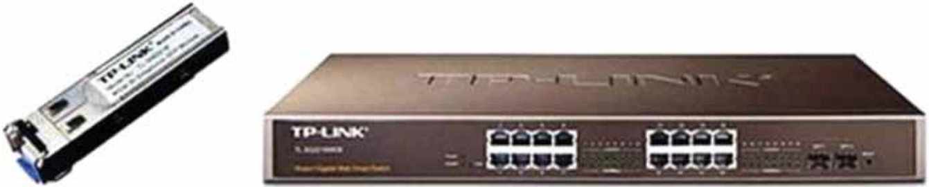
Figure 1. Ethernet switch and optoelectronic transceiver available at the Telecommunications Lab. The transceiver includes a laser diode and a photodetector.
